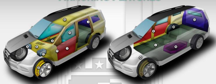
\*\* These schematics represent typical armoring of an SUV. The final vehicle (Toyota Landcruiser 78 Ambulance) may vary depending on the client's required specifications. \*\*
