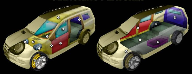
\*\* These schematics represent typical armoring of an SUV. The final vehicle (Toyota Land Cruiser VXR) may vary depending on the client's required specifications. \*\*
