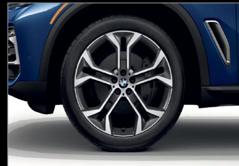
21" Y-spoke orbit grey wheels, style 744, 21 x 9.5 front, 21 x 10.0 rear; and 275/40 front, 315/35 performance 1,2 rear run-flat 1 tires
