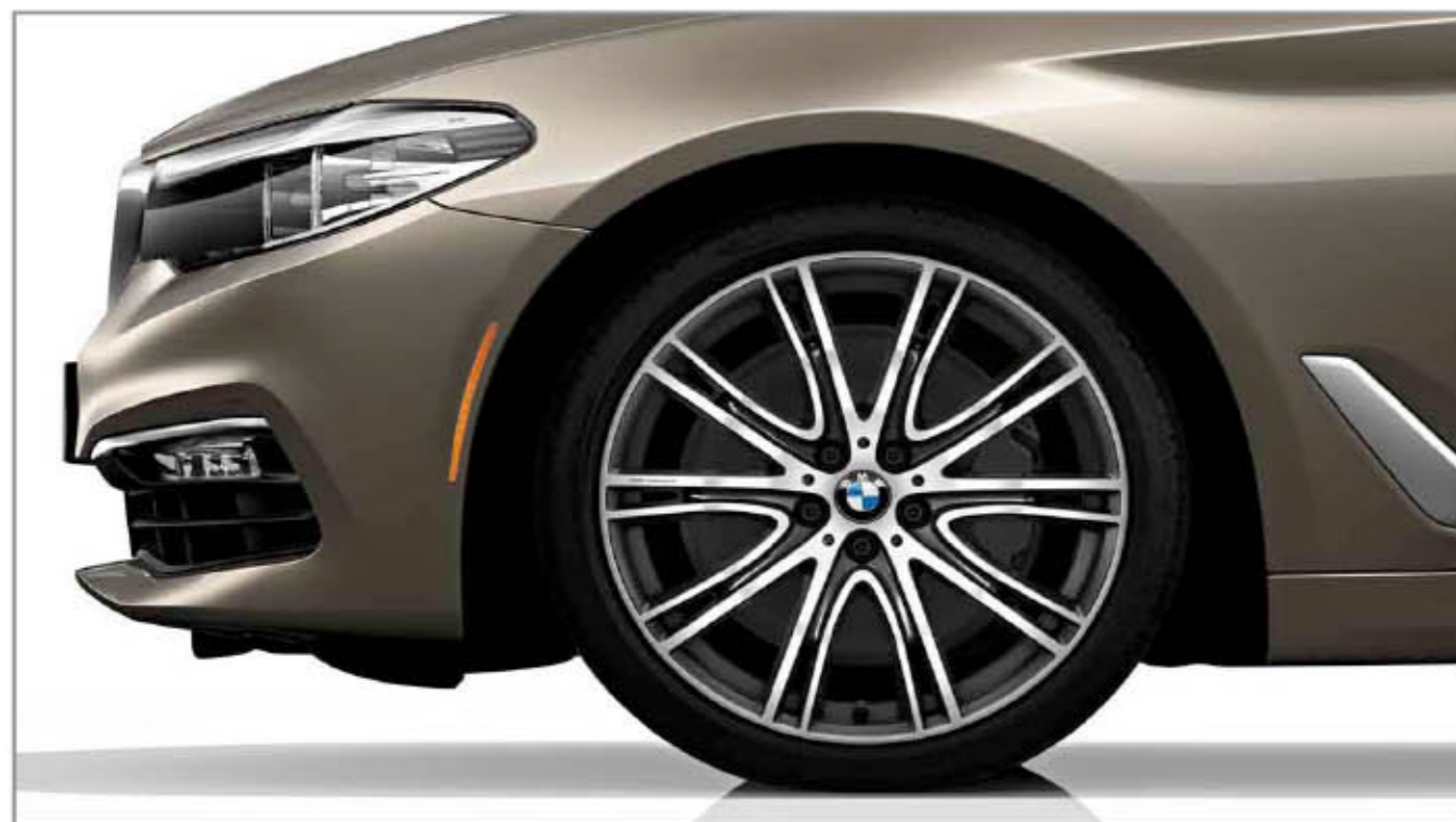
20" V-Spoke wheels, style 759i 20 x 8.0 front, 20 x 9.0 rear; and 245/35 front, 275/30 rear run-flat 3 performance tires 2,4
